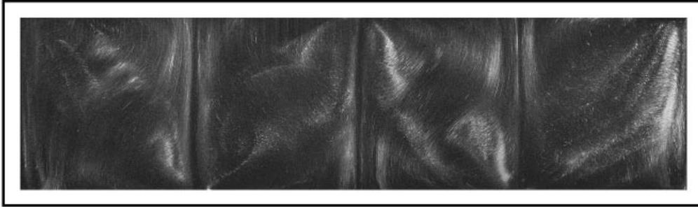
FIGURE 11. Fully developed four-cell state at  $Re = 750$  for symmetrical driving. The moving lid at the bottom border moves towards the observer. The frame indicates the cross-section of the cavity. The light sheet at  $y = 0$  entering from the right side causes a decay of the contrast to the left.
