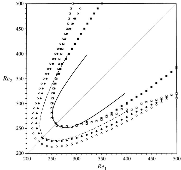
FIGURE 21. Transition boundaries for  $Re_1 \neq Re_2$  and  $\Gamma = 1.96$  (experimental results).  $\bullet$ , two-vortex  $\rightarrow$  cat's eye;  $\circ$  cat's eye  $\rightarrow$  two-vortex;  $\blacksquare$  cat's eye  $\rightarrow$  three-dimensional cells,  $\square$  three-dimensional cells  $\rightarrow$  cat's eye. The theoretical results are included as lines: ---, cat's eye  $\rightarrow$  two-vortex; —, linear instability boundary of the cat's eye flow.
