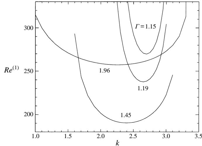
FIGURE 7. Linear stability curves for symmetrical driving:  $Re$  as function of the wavenumber  $k$  for different aspect ratios (as indicated by labels).
