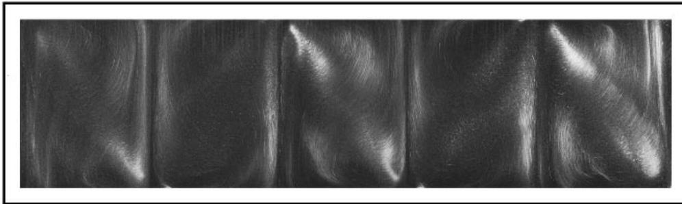
FIGURE 12. Five-cell state at  $Re = 500$  for symmetrical driving. Conditions as in figure 11.
