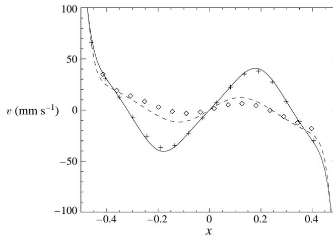
FIGURE 5. Velocity profiles  $v(x)$  of the numerical two-vortex flow at  $Re = 200$  (full line) and cat's eye flow at  $Re = 240$  (dashed line). Velocity data measured by LDA at a distance  $\Delta z = 50$  mm from the endwall are for: +, two vortex,  $Re = 200$ ;  $\diamond$ , cat's eye,  $Re = 240$ .
