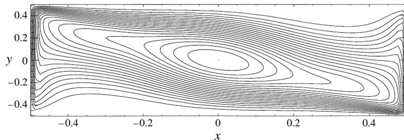
FIGURE 22. Two-dimensional cat's eye flow for  $\Gamma = 3.3$  for symmetrical driving at  $Re = 800$ . The flow is linearly unstable. The  $x$ -axis is scaled by  $d$ .
