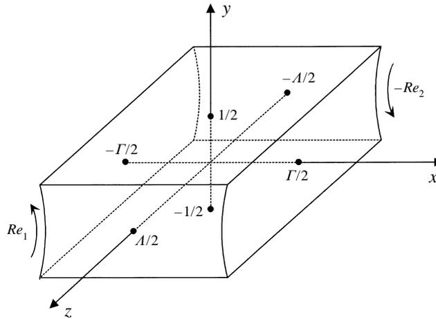
FIGURE 1. Sketch of the cavity and coordinate system.
