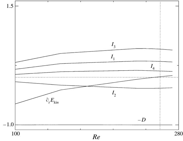
FIGURE 18. Energy balance of the most dangerous mode for the two-vortex state as function of the Reynolds number for  $\Gamma = 1.96$  and  $k = 1.68$  (symmetrical driving). All terms are normalized by the dissipation  $D$ . The vertical line indicates the critical Reynolds number.
