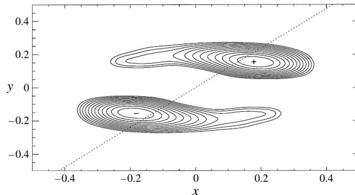
FIGURE 23.  $z$ -component of the vorticity ( $\omega_z$ ) in the plane  $z = \lambda$  (cf. figure 8). The dotted line is the strain direction at the centre of the cavity.
