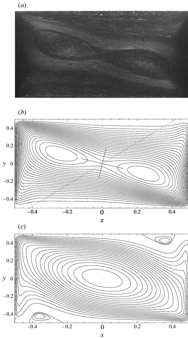
FIGURE 3. Basic cat's eye flow for  $\Gamma = 1.96$  and symmetrical driving  $Re = Re_1 = Re_2$ . (a) Projection of the experimental streamlines at  $z = 0$  for  $Re = 233$ . (b) Numerical cat's eye solution for  $Re = 257$ . The full straight lines represent local coordinate axes and the dotted line is the strain direction at  $x = y = 0$ . (c) Numerical cat's eye solution for  $Re = 800$ . The  $x$ -axes are scaled by  $d$ .
