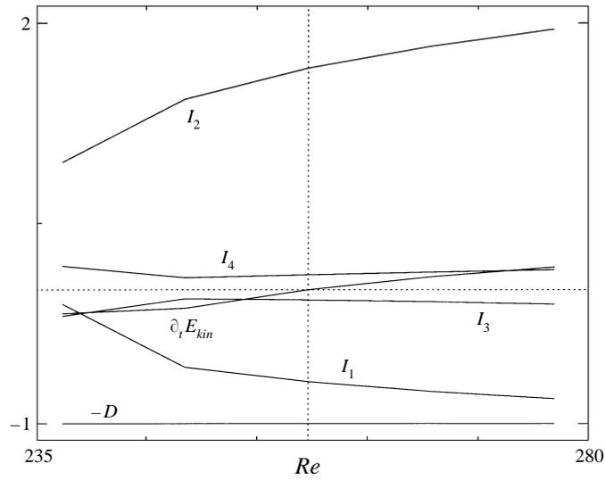
FIGURE 16. Energy balance of the most dangerous mode for the cat's eye state as a function of the Reynolds number for  $\Gamma = 1.96$  and  $k = 2.25$  (symmetrical driving). All terms are normalized by the dissipation  $D$ . The vertical dotted line indicates the critical Reynolds number.
