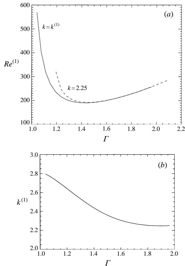
FIGURE 10. Critical curves as function of the aspect ratio  $\Gamma$  for the instability of cat's eye flow (symmetrical driving). (a) Neutral Reynolds number for fixed wavenumber  $Re^{(1)}(k = 2.25)$  (dashed) and critical Reynolds number  $Re^{(1)}(k = k^{(1)})$  (solid). (b) Critical wavenumber  $k^{(1)}$ .
