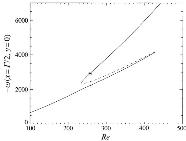
FIGURE 4. Shear stress  $\omega := \partial v / \partial x$  at  $(x = \Gamma/2, y = 0)$  as a function of the Reynolds number for  $\Gamma = 1.96$ . The dashed line indicates an unstable solution. The asterisk and the plus mark the linear stability boundaries of the cat's eye flow ( $Re^{(1)}$ ) and the two-vortex flow ( $Re^{(2)}$ ), respectively.
