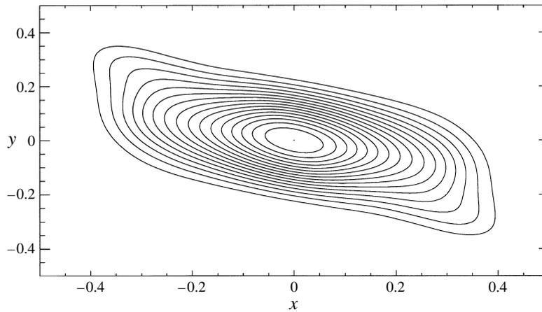
FIGURE 17. Isolines of the local (positive) energy transfer rate from the basic cat's eye state to the neutral disturbance due to the process  $I_2$  shown at the cell boundary  $z = 0$ ;  $Re = Re^{(1)} = 257.2$ ,  $k = k^{(1)} = 2.25$ .
