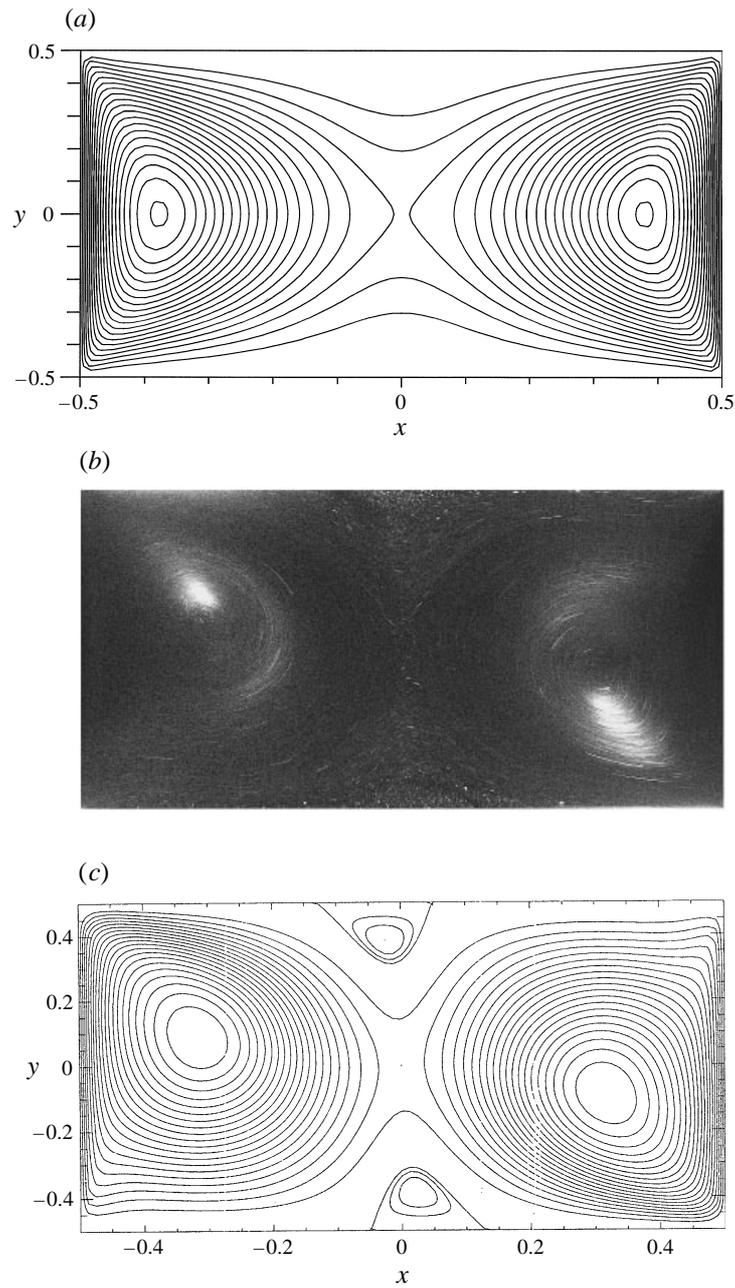
FIGURE 2. Basic flow for  $\Gamma = 1.96$  and symmetrical driving  $Re = Re_1 = Re_2$ . (a) Numerical streamlines of the Stokes flow. (b) Projection of the experimental streamlines at  $z = 0$  for  $Re = 230$ . (c) Numerical streamlines for  $Re = 240$  (The streamlines have been rescaled in the separated region for better visibility.) The  $x$ -axis is scaled in units of  $d$ .
