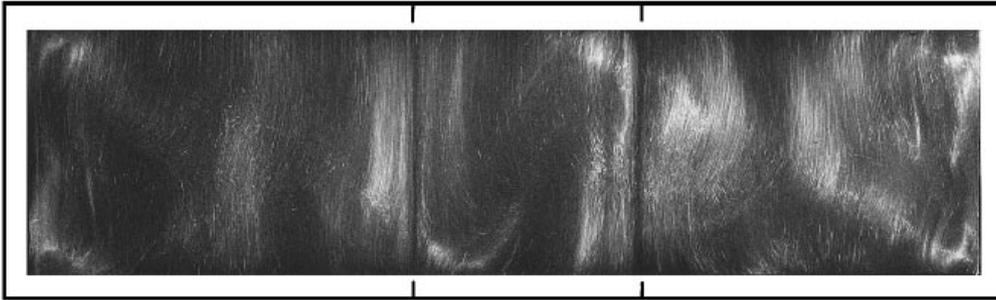
FIGURE 9. A single convection cell at  $Re = 270$  slightly above the critical Reynolds number (symmetrical driving) illuminated by a light sheet at  $y = 0$ . The associated wavenumber is  $k = 2.13$ . The moving lid at the lower border moves towards the observer. The location of the cavity boundary according to  $\Gamma = 1.96$  is given by the frame. The tic marks indicate the cell boundary.
