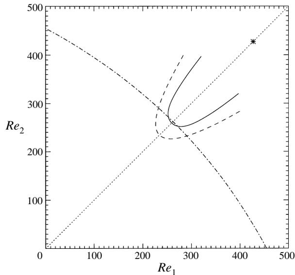
FIGURE 20. Transition boundaries for  $Re_1 \neq Re_2$  and  $\Gamma = 1.96$  (numerical results). Full line: linear stability boundary of the cat's eye flow. Dashed line: lower existence boundary of the cat's eye state. Asterisk: upper existence limit ( $Re^{(0+)}$ ) of the two-vortex state for symmetrical driving. Dash-dotted line: linear stability boundary of the two-vortex flow.
