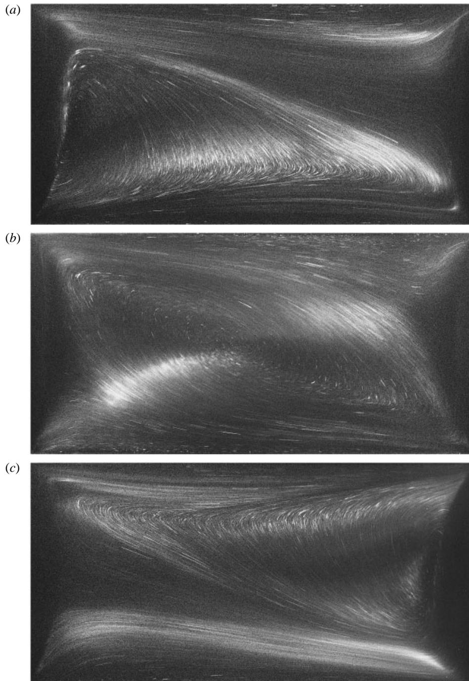
FIGURE 13. Cross-sections through the five-cell state at  $Re = 500$  (symmetrical driving). (a) Cell boundary at  $z = -\lambda/4$ , (b) centre of the cell at  $z = 0$ , (c) cell boundary at  $z = \lambda/4$ . The flow is circulating clockwise.
