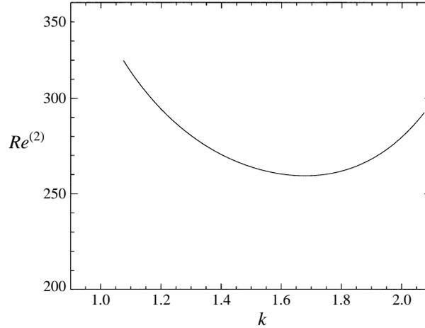
FIGURE 14. Linear stability curve  $Re^{(2)}$  as a function of the wavenumber  $k$  for aspect ratio  $\Gamma = 1.96$  and symmetrical driving ( $Re_1 = Re_2$ ).
