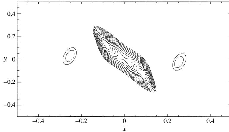
FIGURE 19. The local (positive) energy transfer rate from the basic two-vortex state to the neutral disturbance due to the process  $I_3$  shown on the cell boundary ( $z = 0$ );  $Re = Re^{(2)} = 253$ ,  $k = k^{(2)} = 1.68$  (only the peak level lines are shown for clarity).
