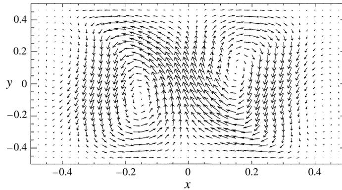
FIGURE 15. Neutral mode of the two-vortex flow state in the  $(x, y)$ -plane, where  $w = 0$  ( $Re_1 = Re_2$ ).
