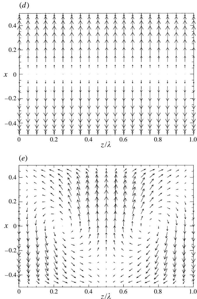
FIGURE 8. Neutral mode of the cat's eye base flow for  $\Gamma = 1.96$ ,  $k = k^{(1)} = 2.25$ , and  $Re^{(1)} = 257.2$  (symmetrical driving). (a)  $u, v$  in the  $(x, y)$ -plane at  $z = 0$ ; (b) contour lines of  $w$  in the  $(x, y)$ -plane at  $z = \lambda/4$ ; (c)  $u, w$  in the  $(x, z)$ -plane at  $y = 0$ ; (d) basic cat's eye flow at  $y = 0$ ; (e) superposition of the basic flow (d) with the disturbance (c) of arbitrary amplitude at  $y = 0$ . The  $x$ -axis is scaled by  $d$ .
